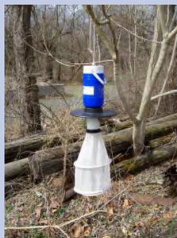
**Light Trap** - collects adult mosquitoes looking for a blood meal. Traps are hung from tree limbs. Dry ice is placed inside the trap as mosquitoes are attracted to carbon dioxide which is emitted from the dry ice.
