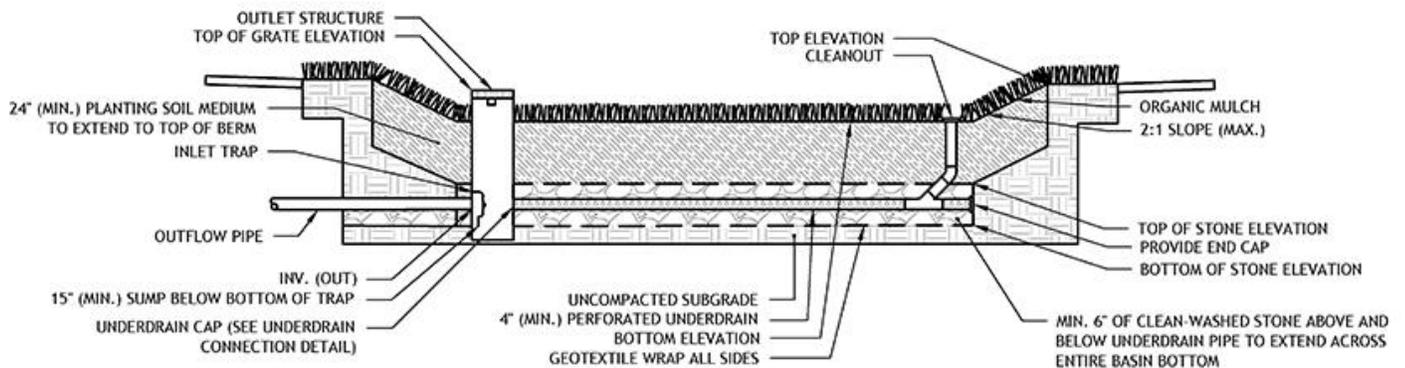
**Underdrain Aggregate Envelope** – A 6-inch stone envelope of AASHTO #57 should be placed around the underdrain. A geotextile (or pea gravel diaphragm) is needed around the aggregate envelope. Note that if the underdrain is placed on the bottom of the BMP, the stone should not be placed throughout the bottom of the BMP, but just in the envelope of the underdrain.
