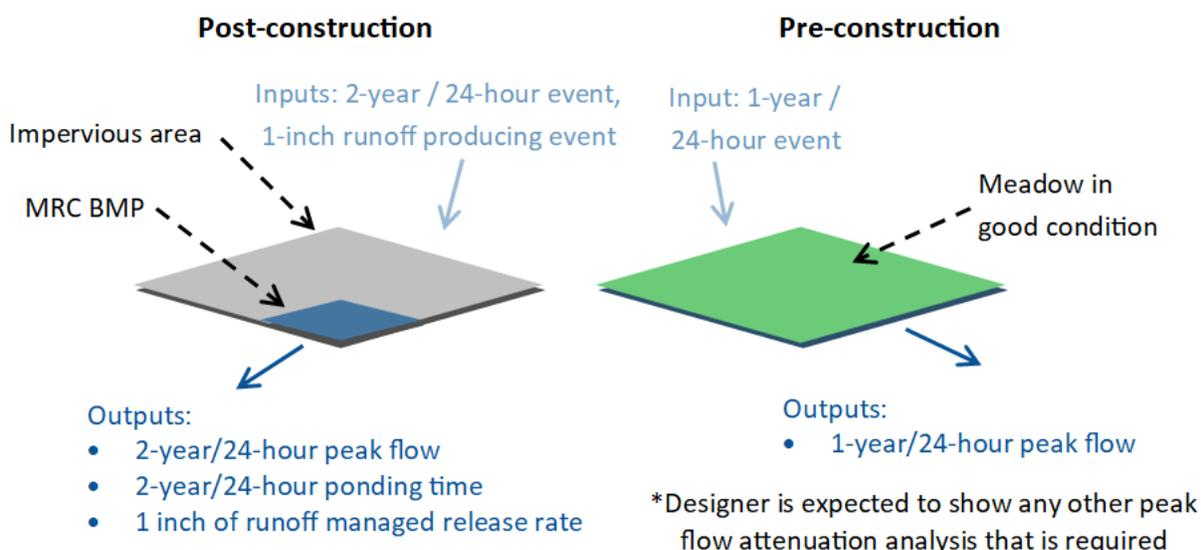
Figure 5: Design Example Schematic
